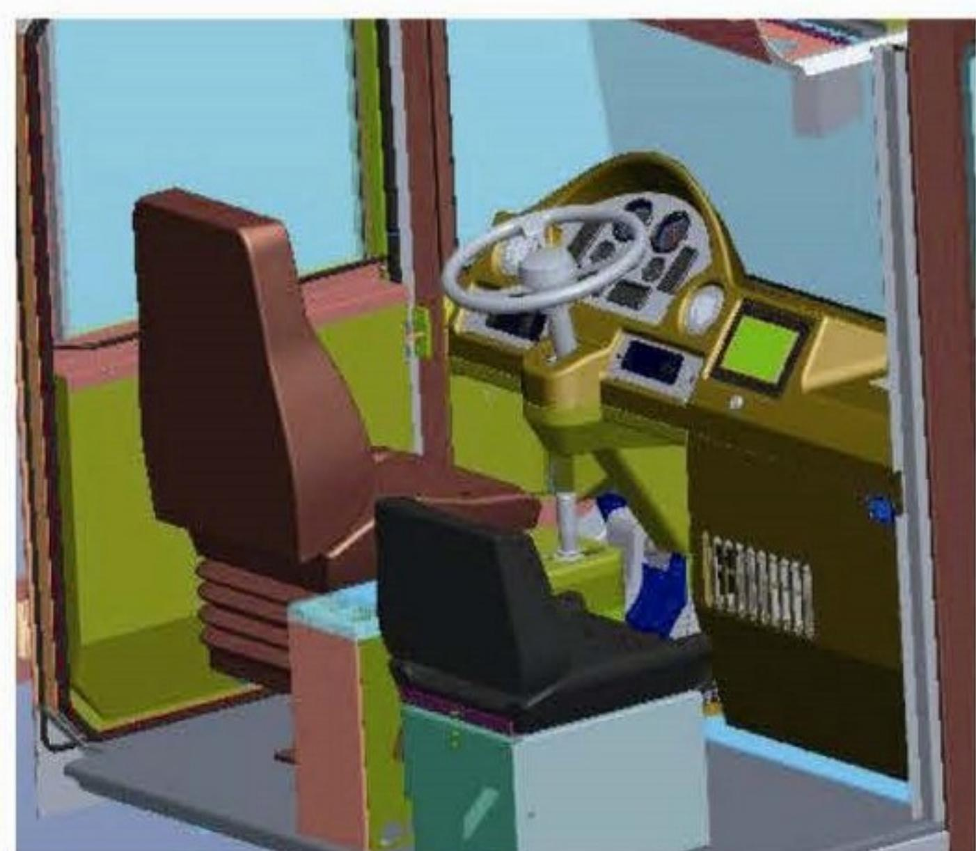
Integral ROPS (Rollover Protective Structure) Cab meets requirements of SAE J 1040. Features include deluxe interior, tinted safety glass, curved windshield for added field of view, tilt and telescopic steering wheel, heater and defroster and pressurized and filtered intake air for driver comfort. Sound exposure is at an Leq (equivalent sound level) of less than 82 dB(A) and is tested per SAE J 1166 MAY90 with doors and windows closed.
