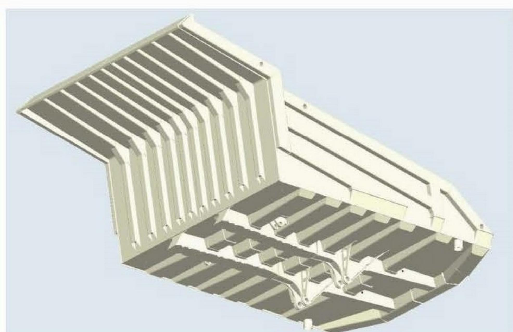
Standard rock body incorporates 3/4" (19 mm) bottom plate with 3/8" (10 mm) side and 1/2" (13 mm) front plate.
