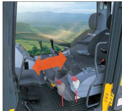
Seat Sliding Amount: 340 mm 13.4", increased 120 mm 4.7"
