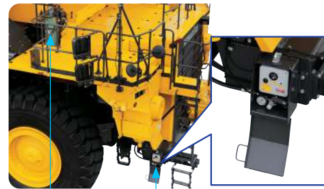
Grease pump and reservoir Refill port
