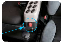
Secondary engine shutdown switch
