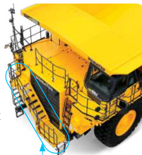
Dimpled slip-resistant plates are used
