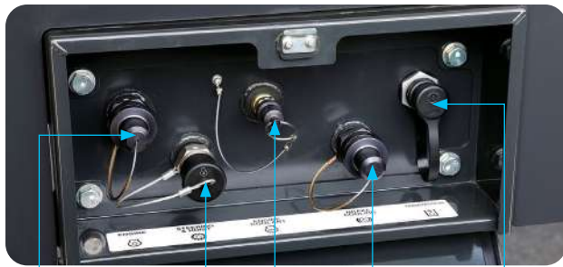
Engine oil Steering and hoist oil Coolant Brake cooling oil Transmission oil
