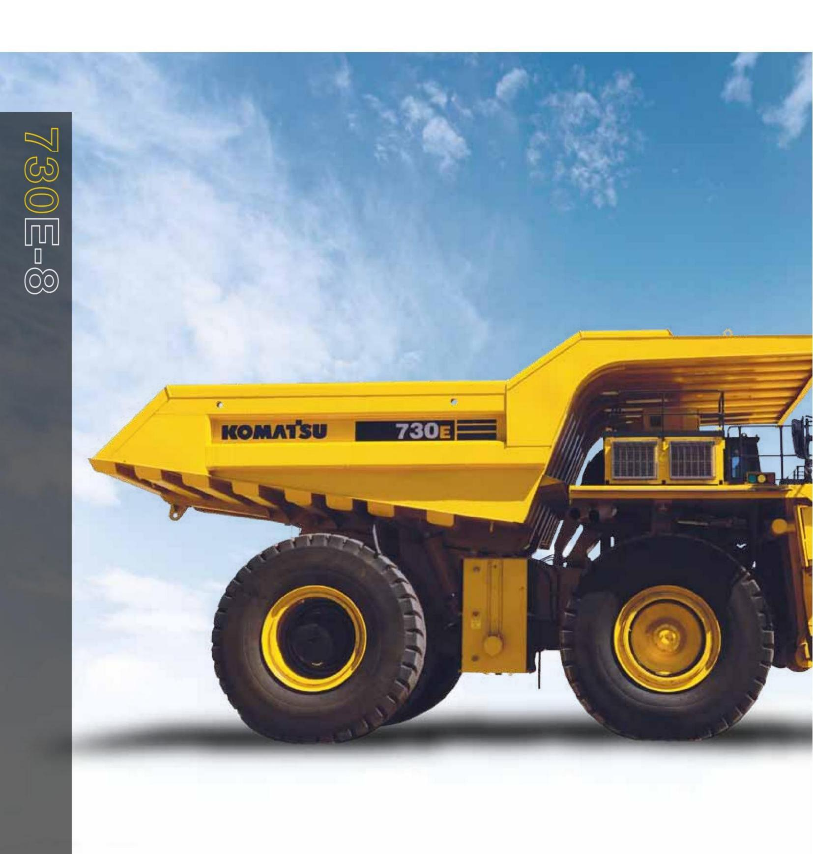
**GROSS HORSEPOWER 2,000 HP** 1492 kW @ 1900 rpm **NET HORSEPOWER 1,884 HP** 1405 kW
